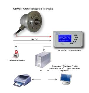
The integrated incremental encoder that is designed for harsh environments links the measured signal to the rotation of the crankshaft. This allows to draw conclusions which crank shaft bearing (or almost any other moving part of the engine) causes the signal.
