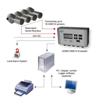
For the case of an alarm, the Evaluator is equipped with two independent relais, so i.e. the shutdown of the engine can be initiated to prevent further damage.
