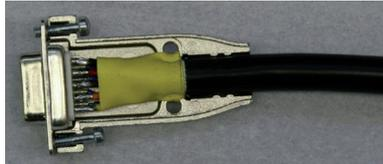
**Fig 8.11. Sub D9 connector after assembly**
