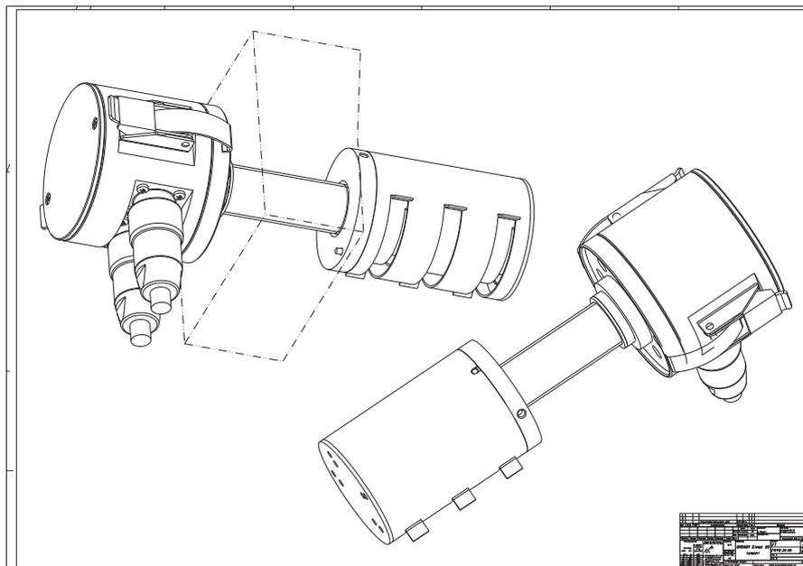
**Fig. 1.6. Installation of SOPS and sensor**
