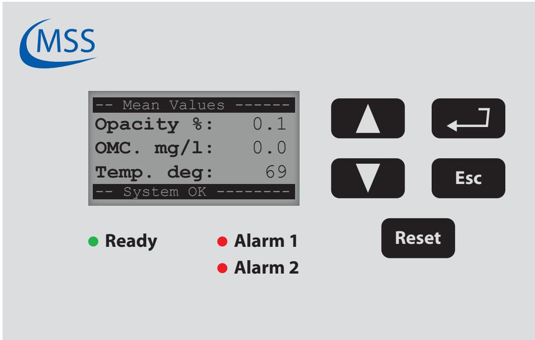
**Fig. 3.1. View of the Evaluator with the default screen**
