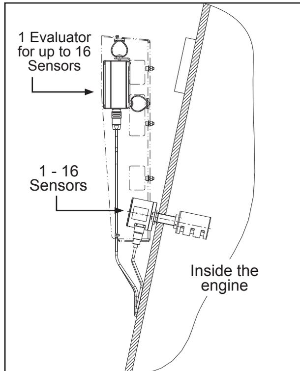
**Fig. 1.1. Exemplary assembly of the GDMS-OMD14 System**
