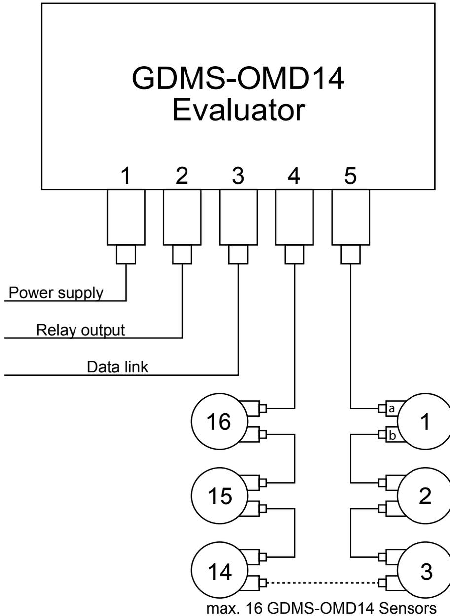
**Fig. 2.2 Principle Connection**
