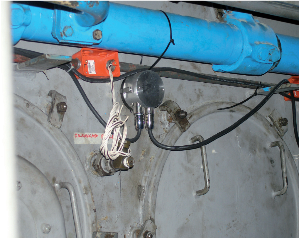
Fig 8.22. Installed Sensor of GDMS-OMDN09 System on a 4 stroke engine
