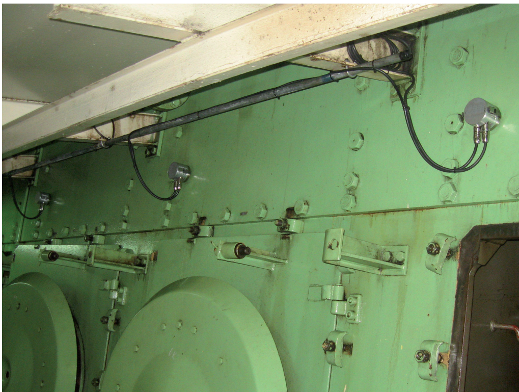
Fig 8.23. Installed Sensor of GDMS-OMDN09 System on a 2 stroke engine
